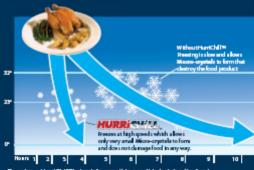
By using a HurriChili<sup>TM</sup> shock freezer, it is possible to bring the food temperature to OT within 240 minutes. Shock freezing is the only system that allows food products to be preserved for weeks or even morths, keeping the initial quality almost intact. Product will not have weight and color loss plus the texture and flavor remain unchanged.
