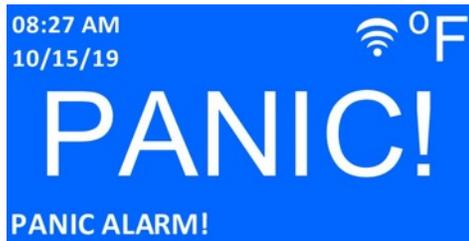
To clear the alarm, push and release the panic button to depress and then press the alarm mute button on the IC+.
