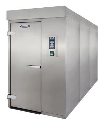
**Shock Freezing:** This cycle is designed to avoid damage to food structure, keeping the food free of large ice crystals. The air temperature is lowered to and held at a range of -25°F to -15°F. The freezing cycle is completed when the food core temperature reaches 0°F.
