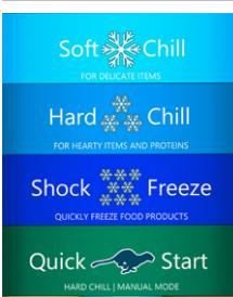
**Soft Chilling:** The air temperature is held in the range of 28°F to 35°F, the cycle is completed when the food core temperature reaches 38°F.
