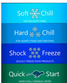
**Soft Chilling:** The air temperature is held in the range of 28°F to 35°F, the cycle is completed when the food core temperature reaches 38°F.
