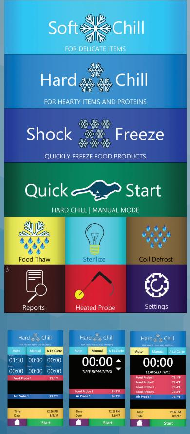
Automatic mode runs the chosen cycle based on input from the food probe. The timer shows elapsed time. Manual mode runs the cycle strictly based on time. An adjustable timer controls the duration of the cycle. A La Carte mode utilizes six timers for management of multiple batches throughout the chilling process.
